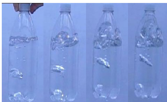
Figure 13: The bubble continues to move upwards even in the free-fall
